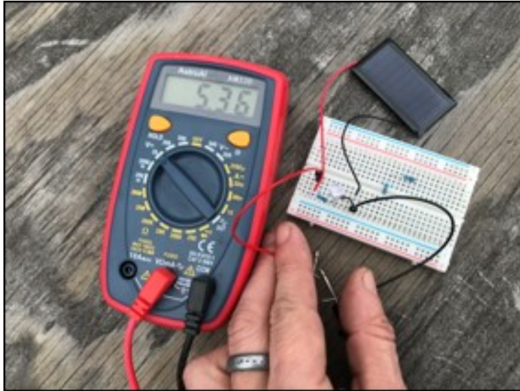
Figure 2: Measuring Voltage in Circuit
